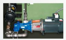
All MSG TURBO-AIR compressors feature a self-contained, low pressure lubrication system.
