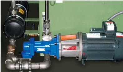
All MSG TURBO-AIR compressors feature a self-contained, low pressure lubrication system.
