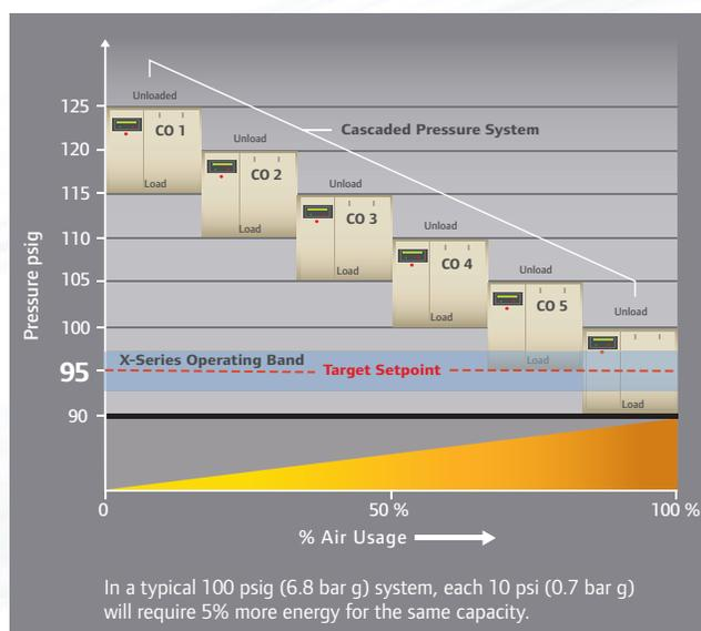
**X-Series Automation eliminates inefficiency by controlling all compressors in a tight pressure band around a single, optimum system pressure, as illustrated by the blue band in the example above.**
