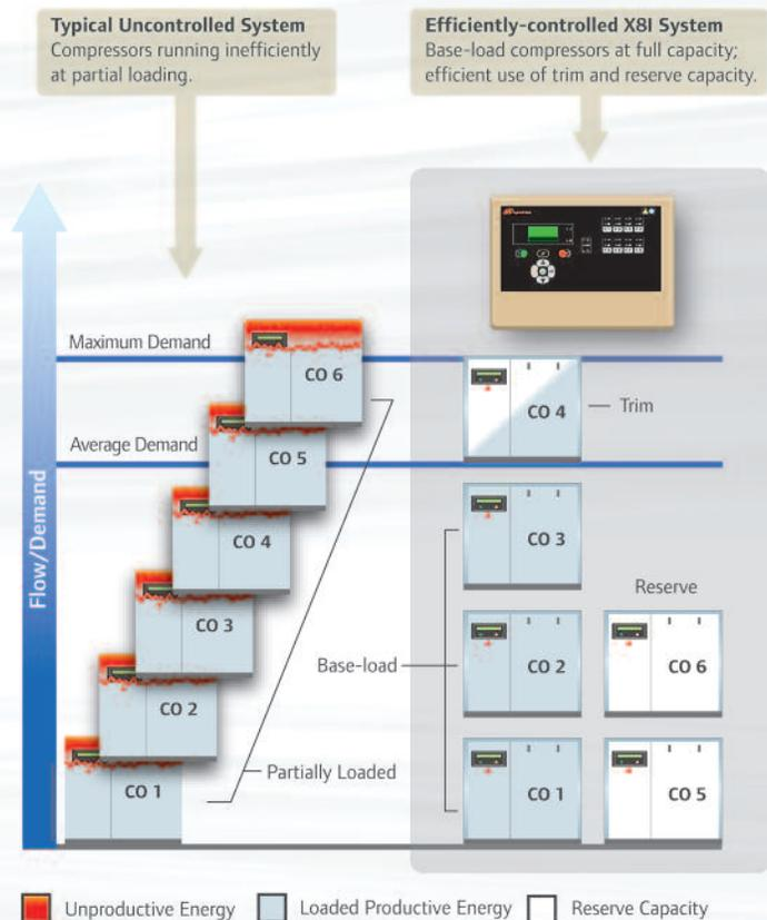
Using the Ingersoll Rand X-Series System Automation to manage a multi-compressor system creates opportunities for significant savings and increased reliability. Keeping compressors off-line until needed eliminates unloaded running costs and creates reserve capacity.
