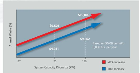
These comparisons show the impact on annual costs of operating your air system at elevated pressures. Compensating for artificial demand is costly work. Considering a system pressure requirement of 90 psig (6.2 bar), the annual operating costs increase by 10% and 20% to accommodate pressure increases of 10 psig (0.7 bar) and 20 psig (1.4 bar), respectively.
