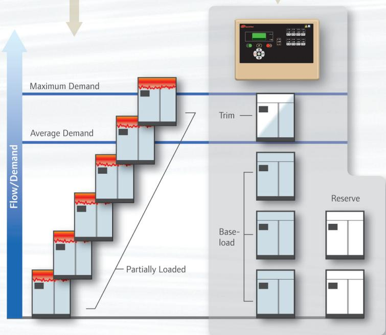
Using the Ingersoll Rand X8I System Automation to manage a multi-compressor system creates opportunities for savings and increased reliability. Keeping compressors off-line until needed eliminates unloaded running costs and creates reserve capacity.
