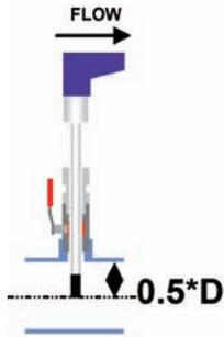
The Airscout probe is shaped to make alignment with the flow direction easy. Alignment "by the eye" is sufficient.
