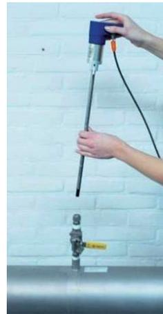
4. Mount the safety line. Hook the safety line up in the ring of the Airscout probe. For extra safety, you can add a luggage strap (like for suitcases).
