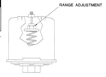
The pressure switch is equipped with a range adjustment control only. No differential adjustment controls are provided.
