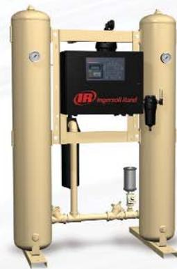
**Heated blower** dryers have a higher initial investment, but with no or little diversion of compressed air from the system for regeneration, they offer significantly lower operating costs.
