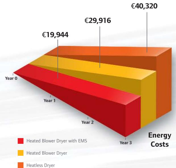
These calculations are approximations based on the following assumptions: Heatless model D3300IL, Heated model D3200IB, 55 m<sup>3</sup>/min, 1,800 CFM, 400 kW Compressor Motor, €0.07 per kW/hr 80 hours per week, and 40 weeks per year.
